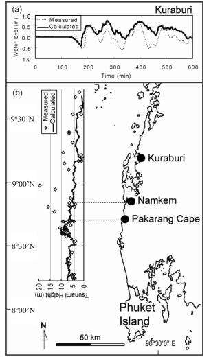
Fig. 6. (a) Comparison between the measured [23] and computed water level at Kuraburi [24]. (b) Andaman coast of Thailand with comparison between measured tsunami heights [12, 13] and computed maximum tsunami heights.
