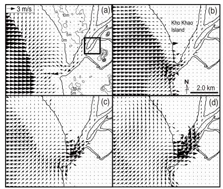
Fig. 8. Snapshots of the computed tsunami current field in the mangrove forest at Namkem at (a) 141 min, (b) 150 min, (c) 153 min, and (d) 156 min after the earthquake. In panel (a), the 5 m interval contour line shows the ground level; the square shows the study area.
