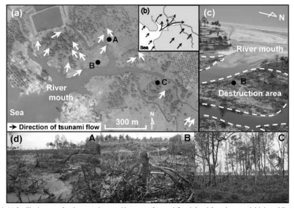
Fig. 4. (a) Satellite imagery after the tsunami event with vectors of tsunami flow inferred from the trapped debris or fallen trees. (b) Trend of the dominant tsunami flow inferred from (a). (c) The destroyed mangrove area photographed from a helicopter (February 2006). (d) Mangrove trees photographed at A, B, and C in Fig. 4a. Photographs A and B show mangrove stumps of destroyed trees; photograph C shows surviving mangrove trees after the tsunami.
